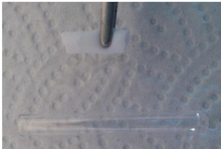
**Figure 4.1 - 13.** Image of centrifuge tube (Ultra-Clear™ 5\*41 mm) and polyacrylamide hydrogel prepared inside the centrifuge tube.
